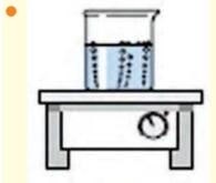
If using a hotplate, ensure that the top plate is larger than the base of the vessel to be heated. Also, neverput cold glassware onto a hotplate which is already well heatedWarm up gradually from ambient temperature.
