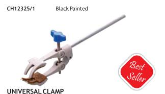
Pressure die cast aluminium alloy, other parts are of plated brass, cork lined, ensures firm grip at all angles of opening, opens upto 90 mm, with  $250 \times 8$  mm nickel plated mild steel rod.
