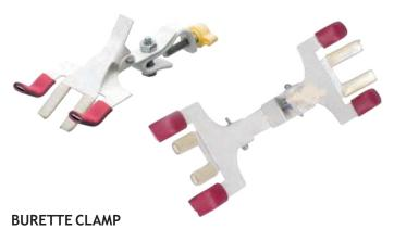
Holds burette in vertical position, die pressed burette clamp of plated steel, jaws having V grooves, with boss to accommodate rods upto 16 mm diam.
